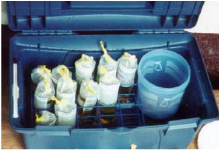
Figure 1; Apparatus used for detection in water of bacteria producing H 2 S.
