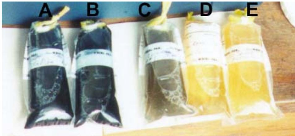
**Figure 2. Typical water samples after incubation to detect bacteria producing H<sub>2</sub>S.**
