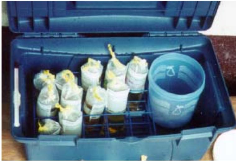
**Figure 1; Apparatus used for detection in water of bacteria producing H<sub>2</sub>S.**
